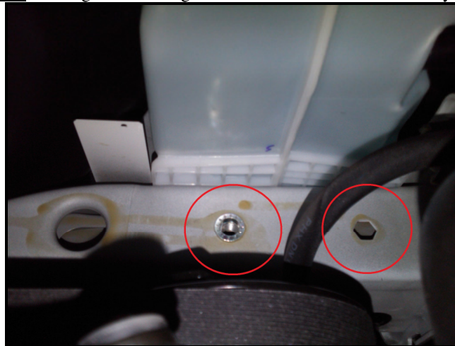
Picture B: Passenger side hexagon holes with one rivet nut already installed.
