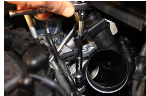
10. Using T30 Torx undo screw at plastic turbo inlet pipe.
