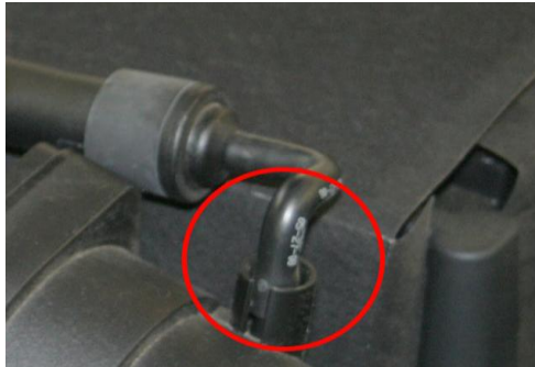
2. Disconnect vacuum hose from air filter box lid.
