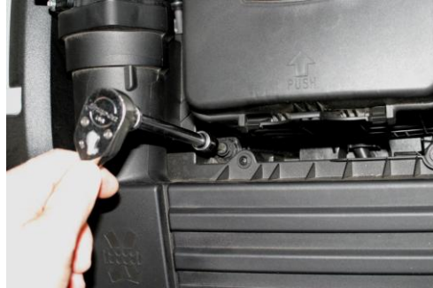
4. Using a 5mm hex key wrench, unbolt air filter box, located on back side.
