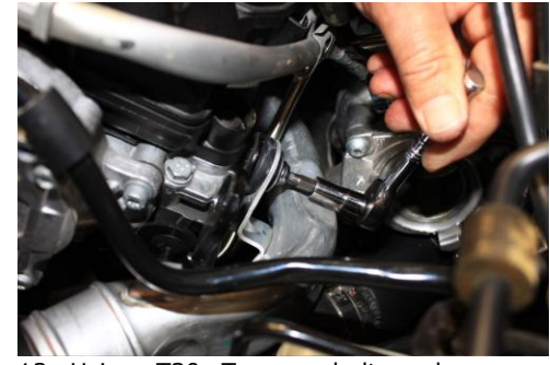
12. Using T30 Torx, unbolt and remove aluminum hot air pipe.
