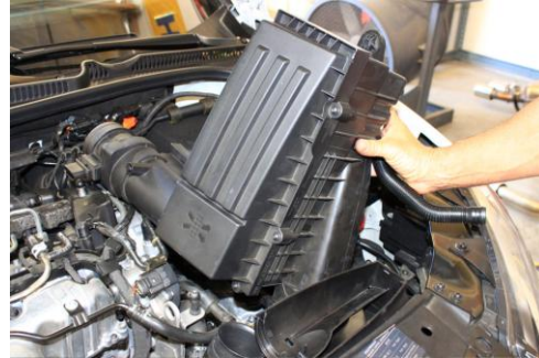
7. Lift off air filter box from rubber grommet mounts, then lift out left side first and rotate intake duct around small coolant hose to remove.
