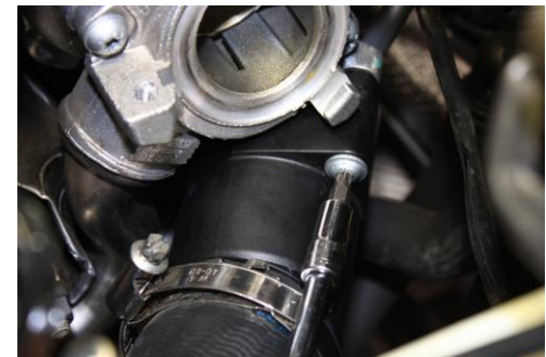
13. Using a T30 Torx remove the (2) screws mounting the plastic turbo discharge pipe to turbo housing.
