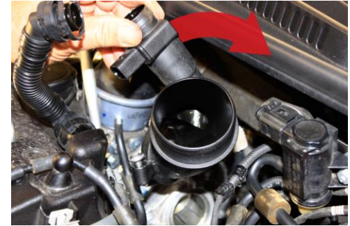
11. Rotate inlet pipe rearward (clockwise) to release from locking tabs.
