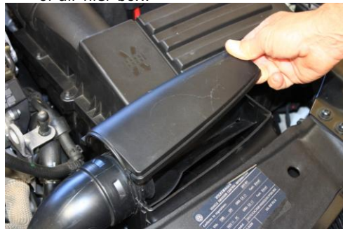
6. Remove cover at intake duct.
