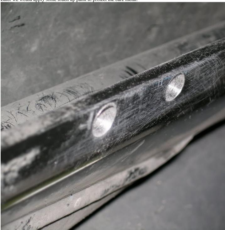
Then we fitted the bar in the c-beam and secured it in place with the clamps. (note the bar isn't quite flush. This was due to the initial alignment of the drill on the first hole. It looks worse than
