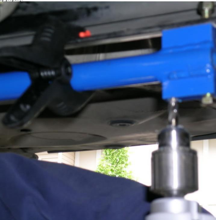
After all four holes were drilled. We sanded the area down to remove burrs and smooth the area.
