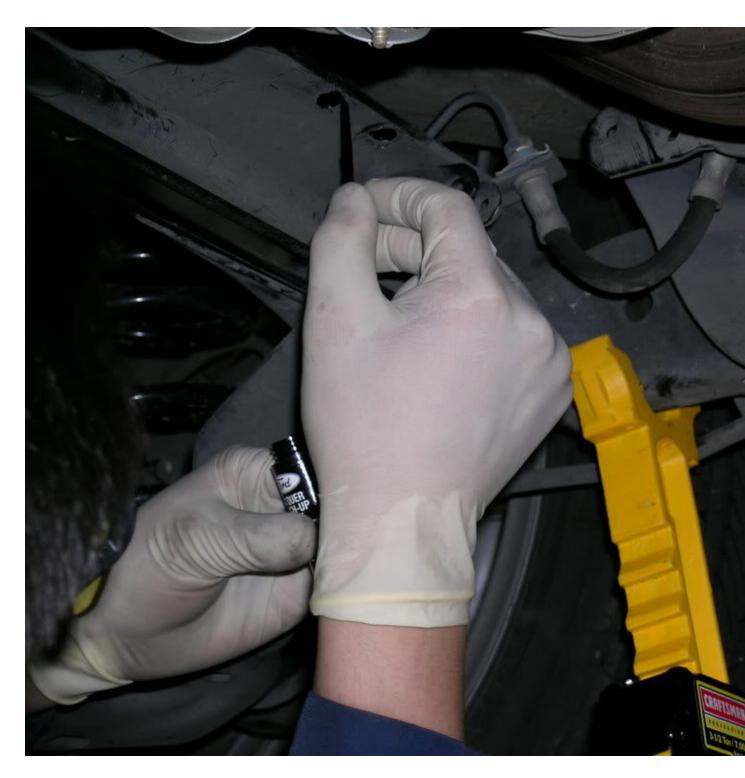
Before installing the bar, Ray insisted on getting every little metal filings out from inside the bar. We kept removing until we couldn't hear the shavings rattling around inside. It was quite a lot. But at least it reduces the rust potential by getting them out of there. Then we applied axle grease to the inside cylinders before placing the bar in the beam. (check out the shavings that just came
