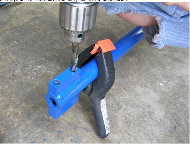
The clamps we were using weren't strong enough to totally hold things in place. So we had to supplement with one of us securing the bar by hand as well while the other drilled. The key to the drilling was to apply as much pressure as possible. But without a lot of room to work in, it
