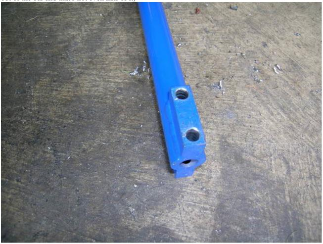
The instructions we were going off of only mentioned inserting the bolts from the top. We found this impossible with the gas tank strap in the way. Maybe this new bar is a different length or earlier vw's had a different strap point. But we had no choice but to insert from the bottom. The only advantage we could see to inserting from the top was if the nyl-nut ever backed out, at least
