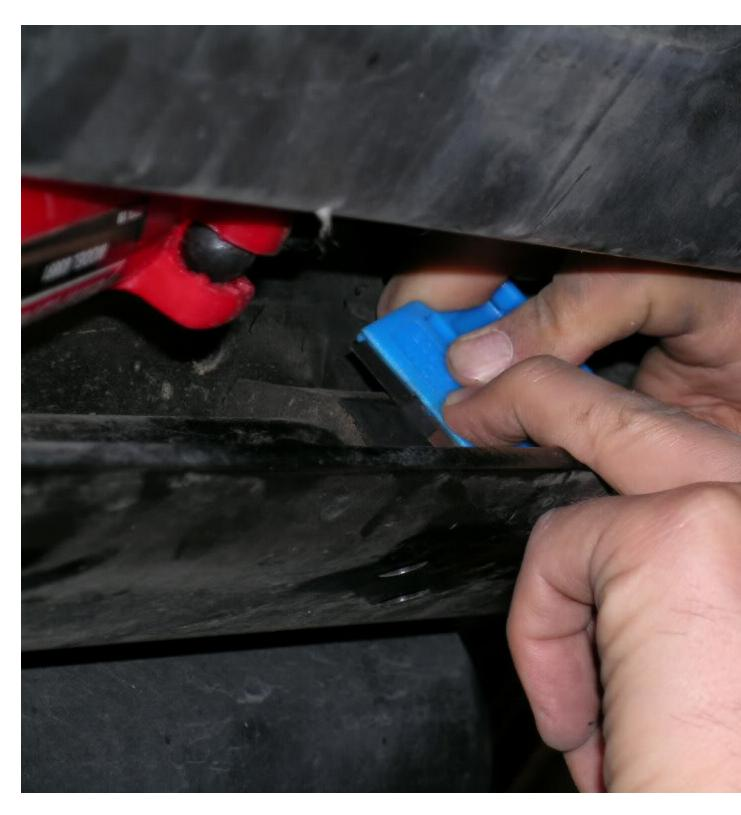
Once enough of the material was cut so the bar would sit nice and flush to the edge of the c-channel, we secured it in place under the beam to drill our first hole. We centered the bar on the
