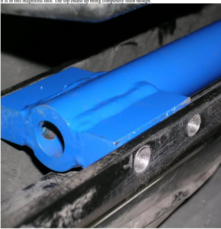
I don't have any pix of the top holes being drilled. But we used the bar in place as a guide/template for the top holes. We decided to combine our efforts by having Ray hold the drill and apply as much pressure as possible. Then I got directly under the drill and pushed upward. It's like 100% exertion by both of us, but we cut our drill time per hole from about 5-7 minutes on the first hole to about 40 seconds on the last two holes. Talk about heat, smoke was coming
