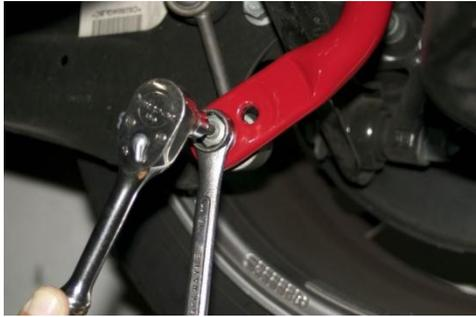
9. Attach end-links to *NEUSPEED* anti-roll bar using original bolts and nuts.
