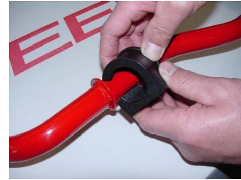
7. Apply silicone grease to the inside of supplied bushings and install on the inside of stop washer on NEUSPEED anti-roll bar.
