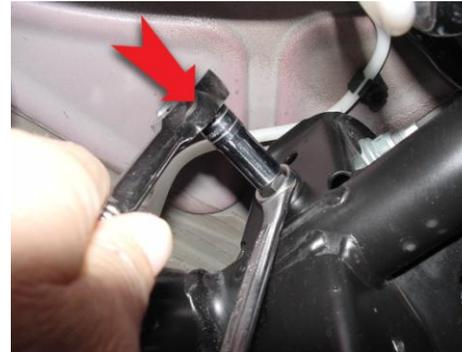
5. Installing Nutsert, hold tool body with 9/16" wrench from turning and push down on ratchet while crimping Nutsert into hole.
