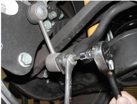
2. Disconnect end-links from original anti-roll bar by securing stud with M6 Triple Square or 5mm hex key wrench and loosening nut with 16mm wrench.
