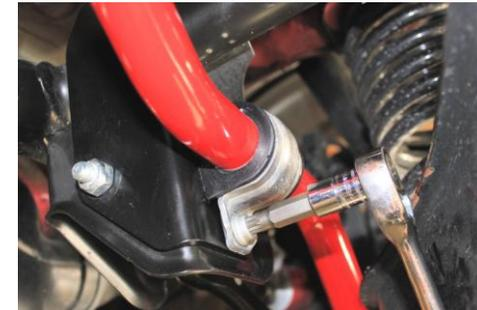
8. Install NEUSPEED anti-roll bar using original clamps and bolts to sub-frame. Torque bolts to 20Nm (15 ft-lbs). **NOTE:** Evenly tighten bushing clamp bolts and sub-frame support bracket nuts and bolts.
