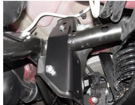
6. Loosly mount Left and Right support Brackets, do not tighten at this time.
