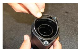
11. Transfer "O" ring from original damper to *NEUSPEED* Damper, then put a little oil on "O" ring.
