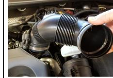
Loosen 7mm hex screw clamp at turbo inlet, then remove plastic air inlet hose.
