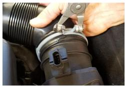
4. Disconnect turbo air intake hose from MAF using spring clamp pliers.
