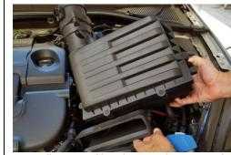
6. Pull up air filter box to disconnect (3) rubber grommet mounts, then remove.
