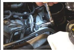
8. Using T30 Torx, unbolt and remove aluminum hot air pipe.
