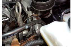
12. Install *NEUSPEED* Damper to turbo, using a 10mm socket and supplied (2) M6x25mm bolts install and tighten.
