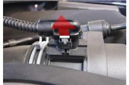
1. Lift up grey locking tab from Mass Air Flow (MAF) sensor electrical connector.
