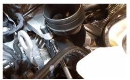
10. Using a T30 Torx remove the (2) screws mounting the turbo damper to turbo housing. Pull damper off turbo, then rearward to disconnect from hose.
