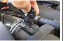
2. Squeeze grey locking tab, then pull to disconnect from MAF.
