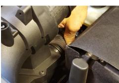
Disconnect hot air duct tube from back side of air filter box.
