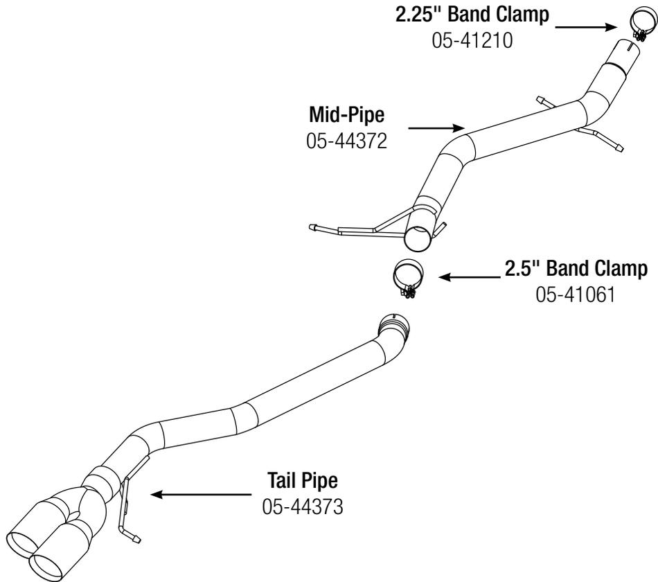
**Step 1: (Read Instructions prior to installation)** Remove your stock exhaust from the rear of your vehicle working your way forward. It will be necessary to cut the pipe to clear the rear axle. Do not cut the pipe after the cat; you will be using this slip connection.
