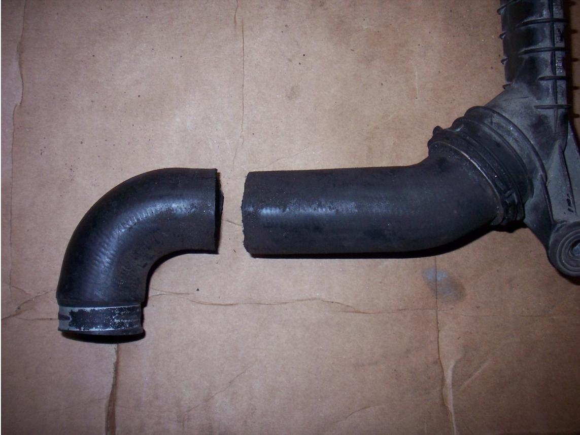
Ensure that any curf (debris created by cutting) have been removed from the air charge hose.
