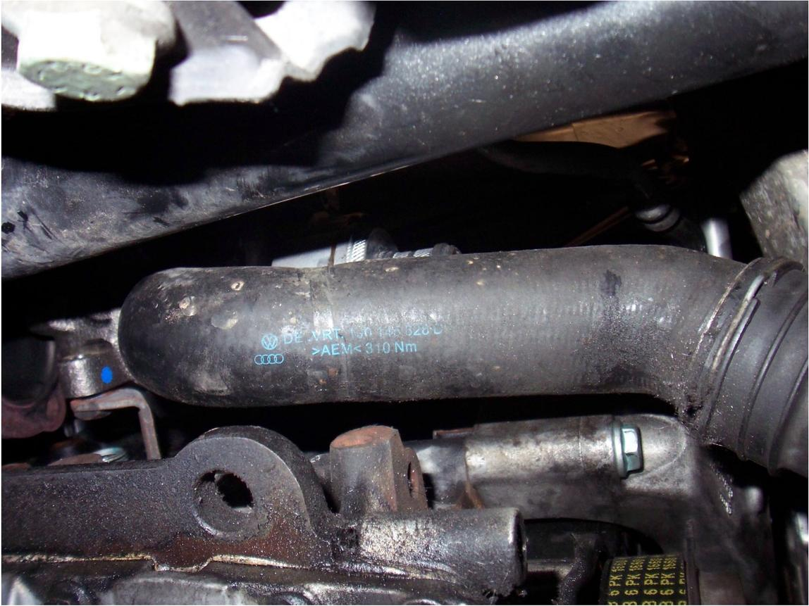
Note that the rubber portion of the air charge piping is too long, and now has an unnecessary 90\* bend. It will be necessary to trim the hose as shown below to achieve proper fitment. Double (or triple) check the location of your cut before cutting.
