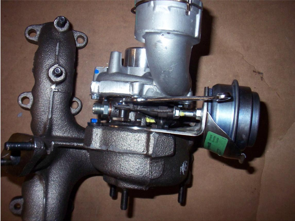
Re-install the housing and bolts with the compressor housing rotated roughly 90\* counter clockwise (when viewing the compressor wheel through the compressor inlet). Note the pictures below for clarification when to re-orientint the compressor housing.
