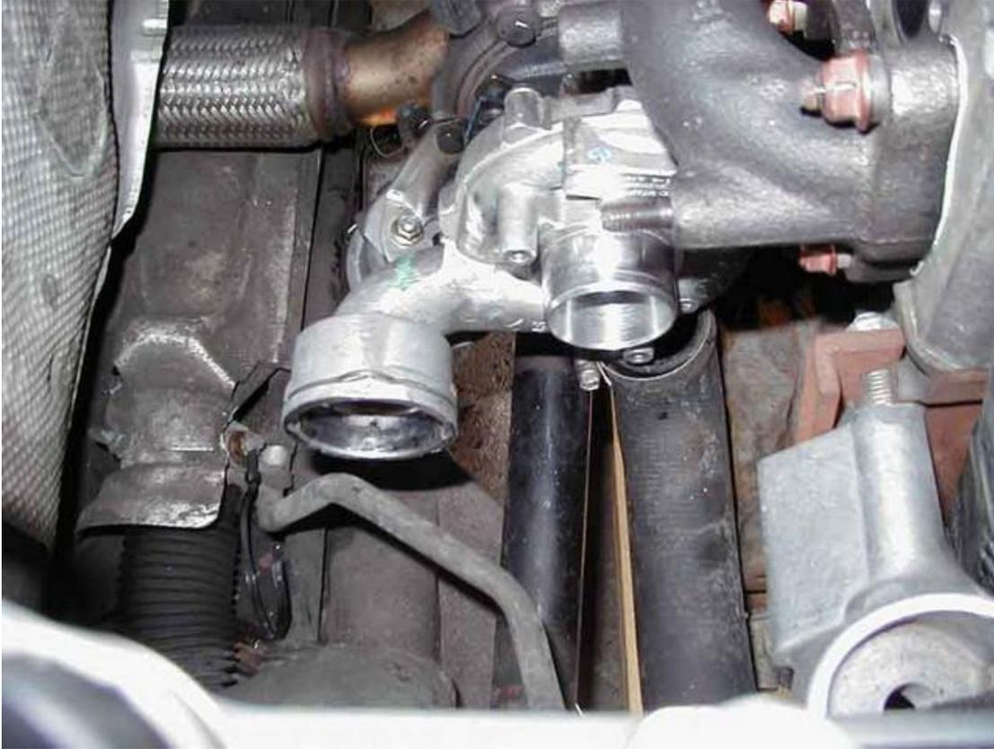
In order to workably install the VNT 17, the compressor housing must be reoriented, AKA 'relocked.'
