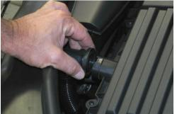
Squeeze collar and disconnect air pump hose from front side of air filter box lid if equipped.
