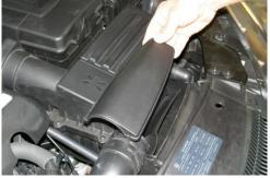
Remove cover at intake duct.
