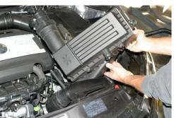
Lift off air filter box from rubber grommet mounts, then lift out left side first and rotate intake duct around small coolant hose to remove. Note drain tubing on bottom right side of air box.
