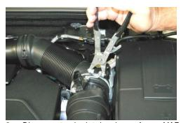
Disconnect air intake hose from MAF using spring clamp pliers.
