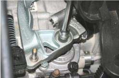
Remove clip on end of shifter cable and lift off. Unbolt gear selector lever from selector shaft using a 13mm socket – now remove lever (rock lever back and forth while pulling up).
