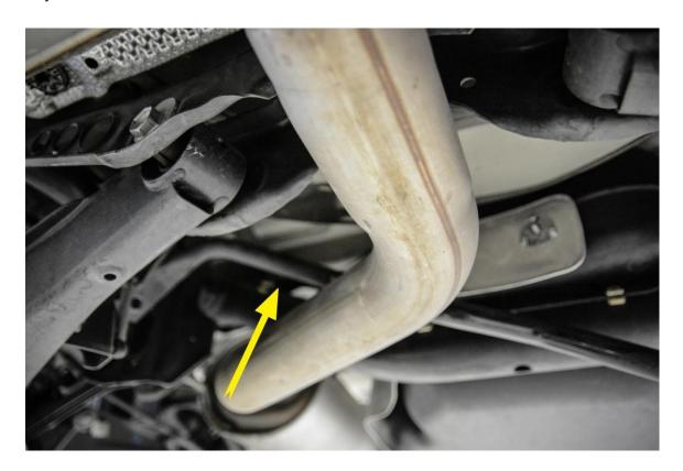
**Step 6** – Using the same technique, rotate and position the new 034Motorsport Mk5/Mk6 FWD rear sway bar underneath the car. **Careful** not to hit the exhaust when getting the sway bar in position.
