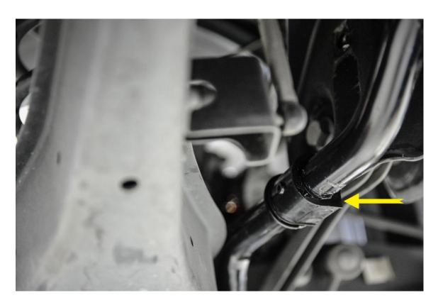
**Step 8** – Prepare to install the Billet Aluminum Sway Bar Mounts, and apply a small amount of blue loctite to each of the supplied M8 bolts.
