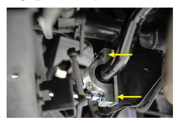
**Step 10** – With the sway bar in place, install the supplied M10x65 bolts and nylock nuts to the factory rear end links using a 15mm and 16mm wrench. Torque the stock hardware to 35 Nm.
