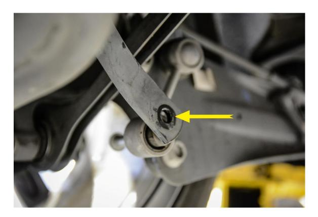
**Step 4** – Using the 10mm Triple Square, remove the two M8 Bolts securing each of the factory rear sway bar mounting brackets to the subframe.
