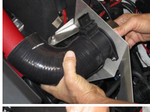
17. Install 90° silicone hose onto MAF. NOTE: Use silicone spray to ease install. Slide the two supplied #48 hose clamps onto silicone hose and then connect to intake pipe. Now position clamps and tighten.
