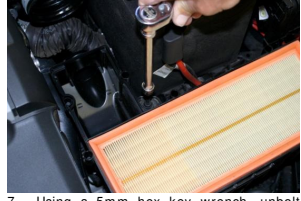
7. Using a 5mm hex key wrench, unbolt lower air filter box, located on back side.
