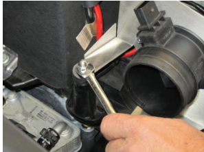
15. Install and tighten acorn nut using an 11mm wrench.
