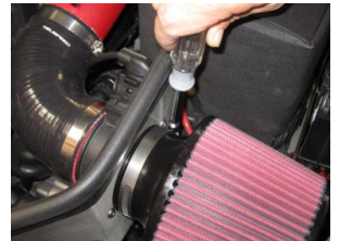
23. Attach and tighten NEUSPEED filter. Position NEUSPEED logo on end of filter horizontally.
