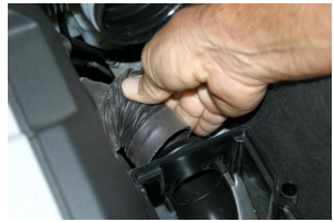
5. Disconnect hot air duct from back side of air filter box.
