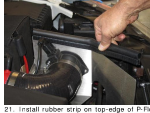
21. Install rubber strip on top-edge of P-Flo bracket.
