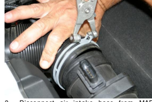
3. Disconnect air intake hose from MAF using spring clamp pliers.
