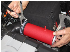
16. Install intake pipe with port closer to the front and positioned at 1 o'clock.
