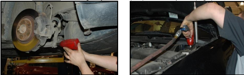
Picture A: Removing sway bar bolts (Left) and strut cap bolts (Right).
