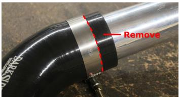
Tightnen a clamp around the silicone leaving only the amount you are wanting to remove at the end.
