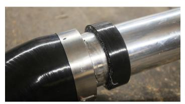
Once you have cut all the way round make sure you can seperate the silicone off cut. You can then remove the clamp and silicone leaving you with the finished shorter silicone.
