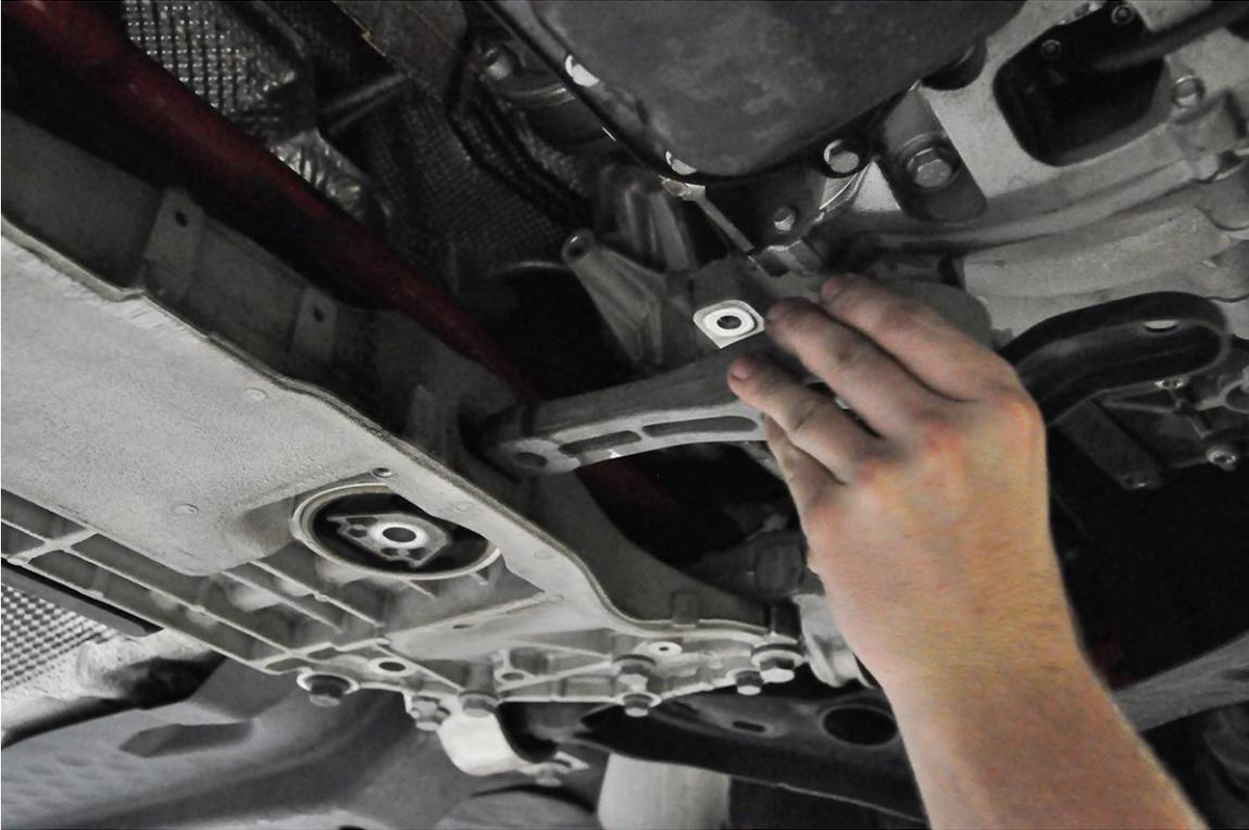
**Step 4** – Install the shiny new 034Motorsport Dogbone Mount into the subframe, and start threading in the factory bolt (with Blue Loctite) to keep it in place. Make sure the spacer is on the top of the dogbone mount, between the spherical and the transmission, and the small bracket is at the bottom, as pictured below. The 034Motorsport logo should be facing down, so we get some free advertising to small critters that might crawl underneath your car.
