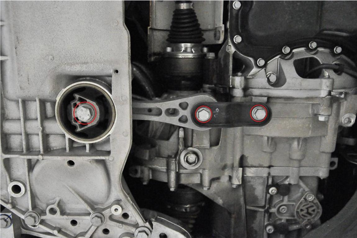
**Step 2** – Using the 16mm socket, remove the two front bolts from the dogbone mount, and using the 21mm socket, remove the rear bolt at the subframe. Let the feeling of accomplishment overcome you.
