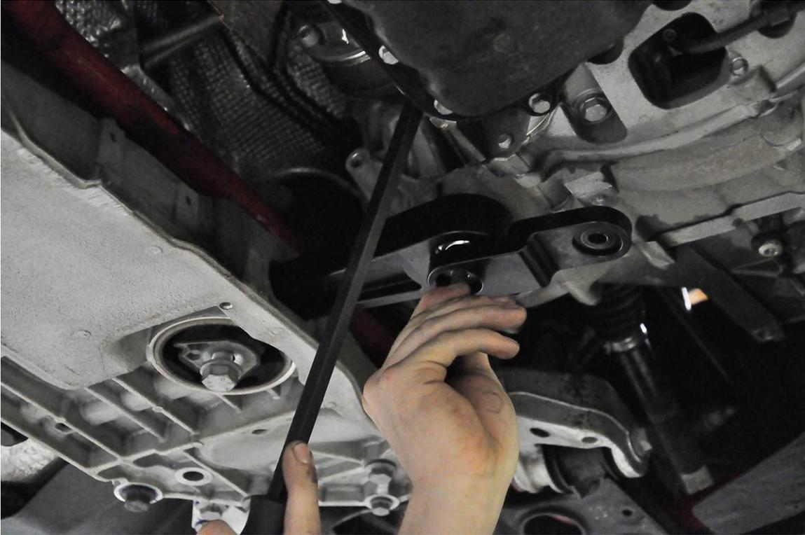
**Step 6** – Torque the factory rear dogbone bolt (with Blue Loctite) to 100 Nm. Torque supplied 17mm bolts (with Blue Loctite) to 45 Nm.
