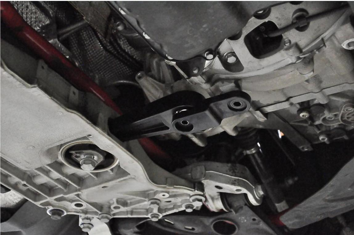
**Step 5** – Using a pry bar, align the bolt hole on the transmission with the center hole in the 034Motorsport Dogbone Mount. Loosely thread in the supplied M10x75 bolt (with Blue Loctite) by hand to keep it in place. Install the supplied M10x35 bolt (with Blue Loctite), securing the front bracket to the transmission.
